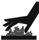
Some of the engine and Sail-Drive surfaces become very hot during operation and shortly after shut-down. Keep hands and other body parts away from hot surfaces.
