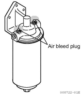
4. Fill the fuel with the fuel priming pump.
