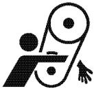
Stop the engine before you inspect it. If you have no choice but to inspect the engine while it operates, keep your hands, other body parts and clothing away from rotating parts.
