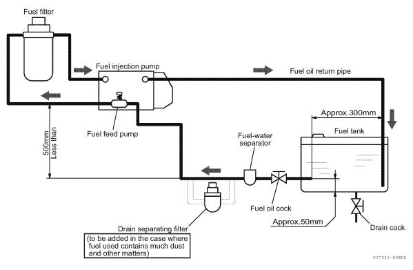
Check the piping between the fuel tank and the engine as illustrated above.
