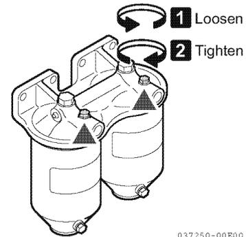
3. Loosen the air vent plug on the top of the fuel filter.
