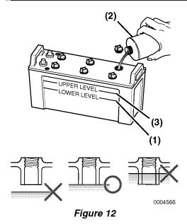
Note: The maximum fill level is approximately 10 to 15 mm (3/8 to 9/16 in.) above the plates.
