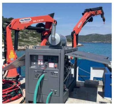
Custom made to suit the netcleaners needs. Stand alone, complete solution with water cooled marine diesel engine, very good service accessibility, low fuel consumption!
